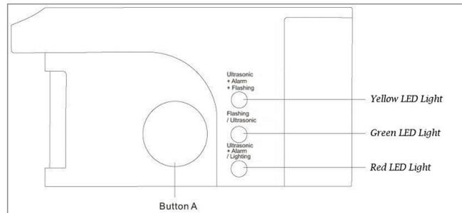
(c) briefly press button A to set the first device operating mode (each successive button stroke enables you to switch between the two following modes)
